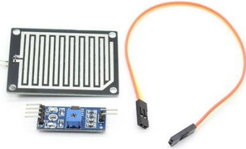
Figure 8: Water Conductivity Sensor
