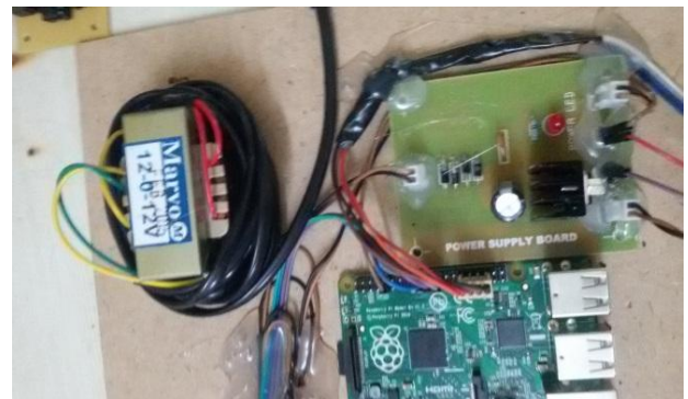
Figure 19: Power Supply Interface
