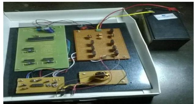
Fig. 15. Prototype of PMSM Fed by Z-Source Inverter
