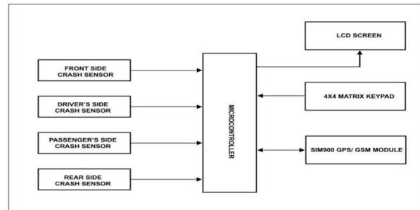
Fig. 2. Block Diagram of Accident Emergency SMS Tracking System
