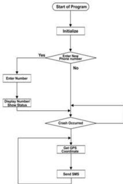
Fig. 4. Program Flow Chart of Accident Emergency SMS Tracking System
