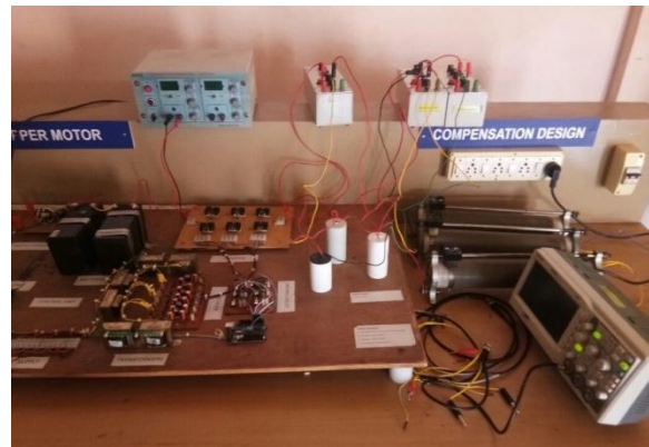
Fig. 4.1 Experimental Setup of Arduino Base Three Phase Inverter With RC Filter
