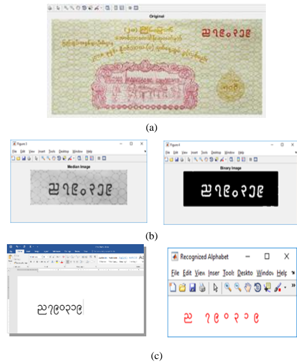
Fig. 7. (a) Original Image, (b) Pre-process Result, and (c) Recognized Number
