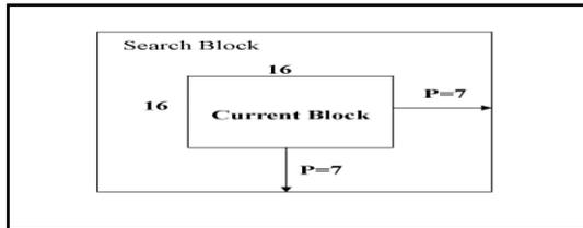
Fig. 1. Block Matching a macro block of side 16 pixels and a search parameter p of size 7 pixels [6].
